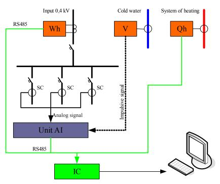
*Pic. 5. The structural scheme of a system of controlling and managing energy consuming:*
